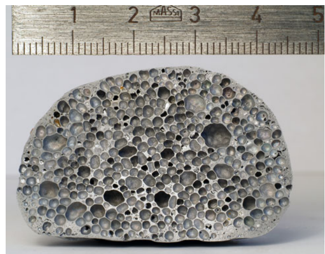
Fig. 12 Photographic image of a foam made from AlMg4Si8 alloy, showing a uniform pore structure
